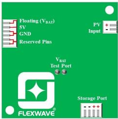
Please make sure storage port is well connected to keep system work stably
